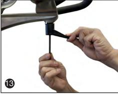
Step 14: Loosen the L-Handle counter-clock wise. Slide the Handlebars back and forth, making sure they can move freely and be locked into all positions on the Bottom Slide.
