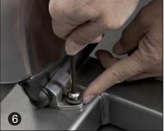
**Step 7:** By not fully tightening the bolts, the brackets allow the tube to move left to right to some degree. Center the tube with as much clearance as possible from the flywheel, then fully tighten all the bolts. Make sure the tube is centered over the flywheel. The flywheel must be completely hidden behind the tube as shown below.
