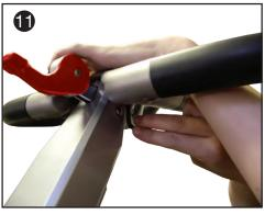
Step 2: Tilt the handlebar assembly slightly to place the socket head cap screws (M8x1.25 X 12 SS) into the mounting holes (Fig. 11). Once each screw has been started, place the palm of one hand on the center of the handlebar pressing firmly and evenly onto the handlebar post. With the other hand tighten each screw with the Allen wrench until the head of each screw just makes contact with each hole. Now tighten each screw evenly.
